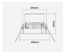
Integrated LED Luminaire F28100RC-d-24 °
